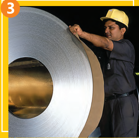
3 Wrapping the coil in HDPE fabric Laminated VCI paper & metal sheet
