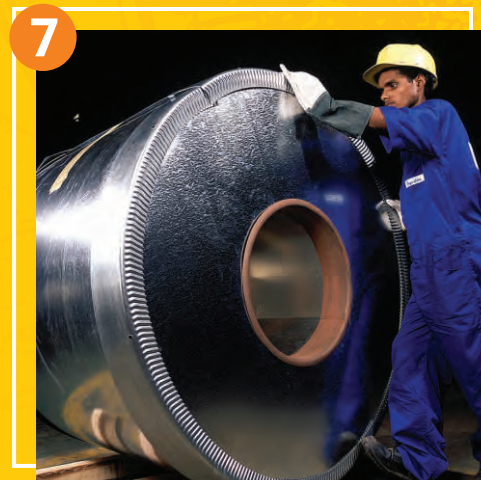
7 Fixing metal protectors on the sides and metal edge protectors on ID & OD straps
