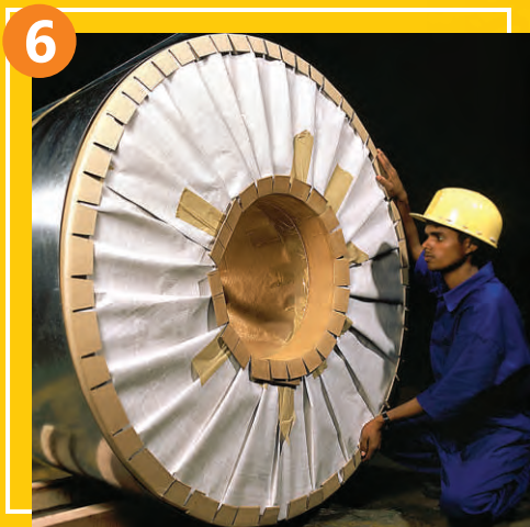
6 Fixing the paper edge guard on the OD and ID
