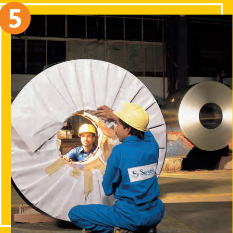
5 Tucking the VCI paper in to cover the edges and ID
