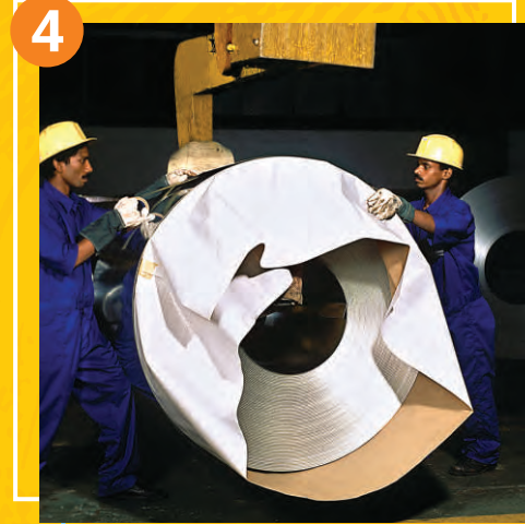
4 Strapping around the OD to hold the VCI paper & metal sheet on the coil
