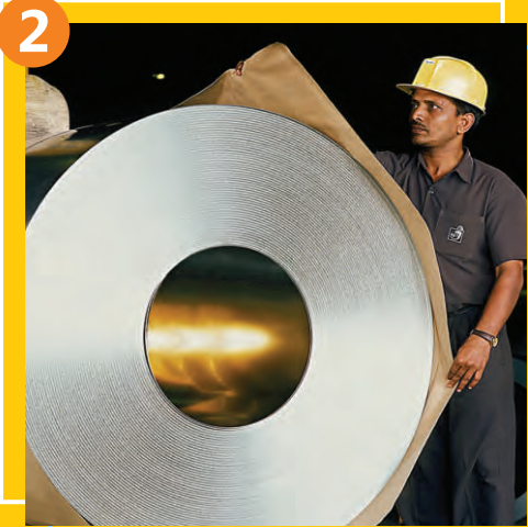
2 Placing the coil on HDPE fabric laminated VCI paper & metal sheet
