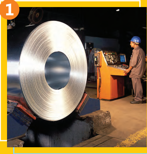
1 Fresh edge slitted coils from mill VCI oil when sprayed on the edges protects against moisture & acid fumes
